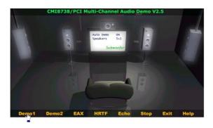
2. Move mouse to the upper half of screen (blue words) until it turns to palmation. Click mouse left key to display the advanced setting screen.
