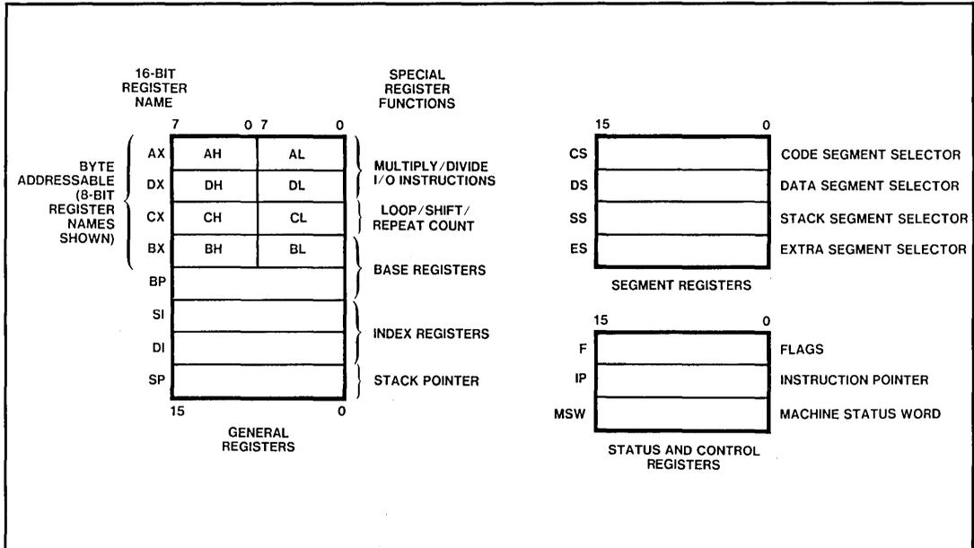
Figure 2-4. IAPX 286 Base Architecture Register Set
