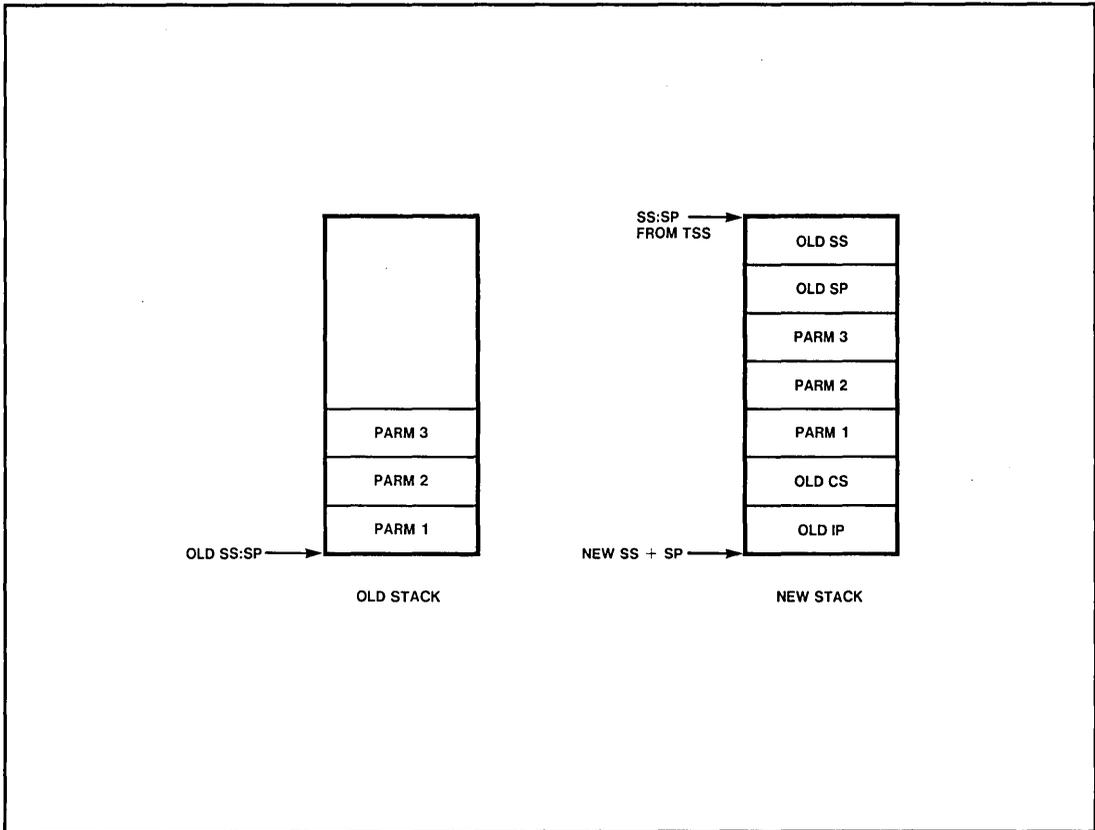
Figure 7-12. Stack Contents After an Inter-Level Call
