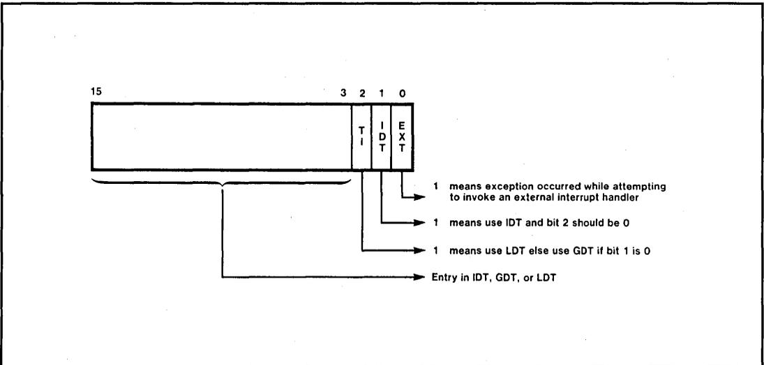
**Figure 7-5. Error Code Format (on the Stack)**
