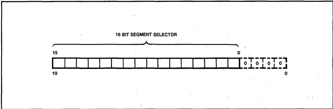
Figure 5-1a. Forming the Segment Base Address
