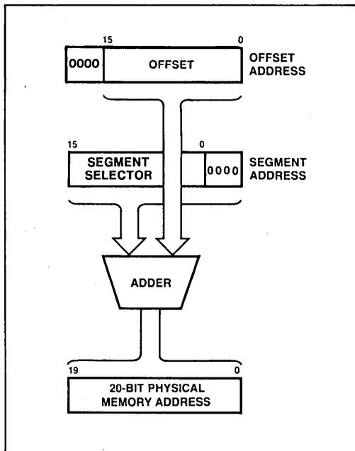
Figure 8. iAPX 86 Real Address Mode Address Calculation
