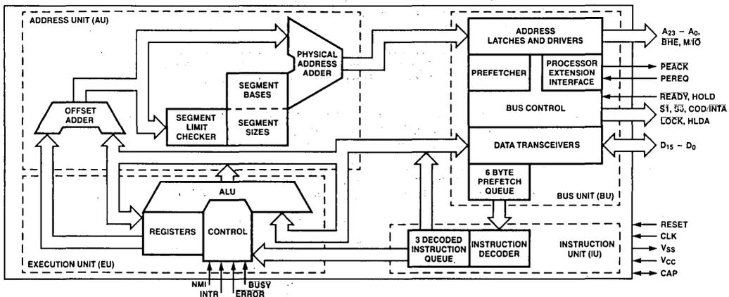
**Figure 1. 80286 Internal Block Diagram**
