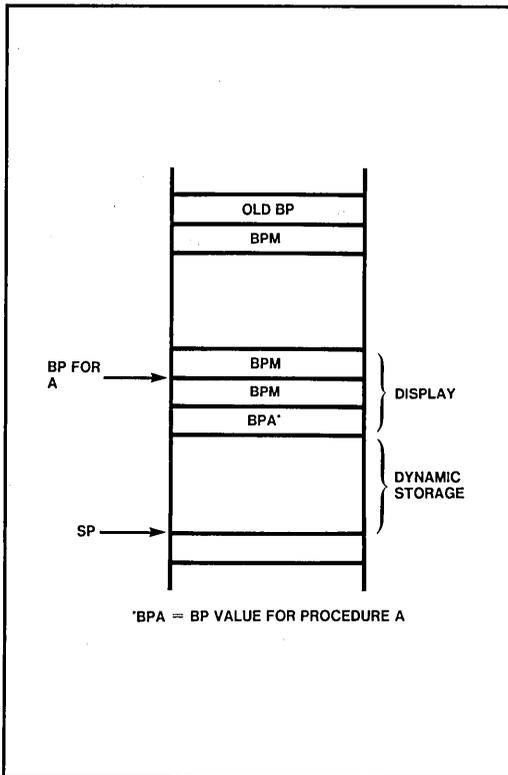
Figure 4-2b. Stack Frame for Procedure A
