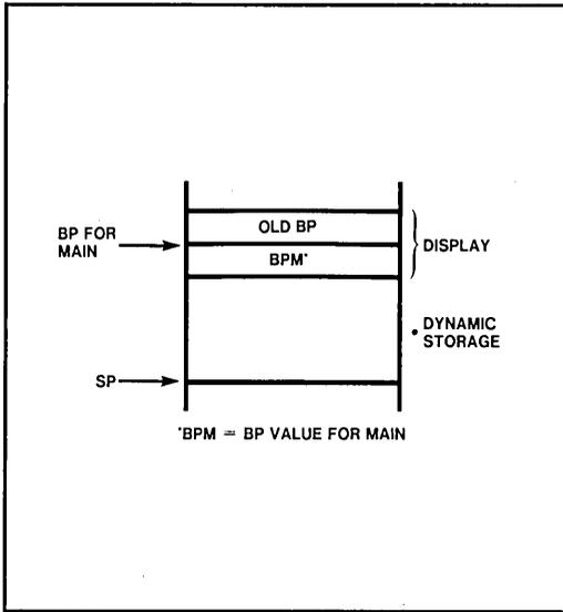
Figure 4-2a. Stack Frame for MAIN at Level 1
