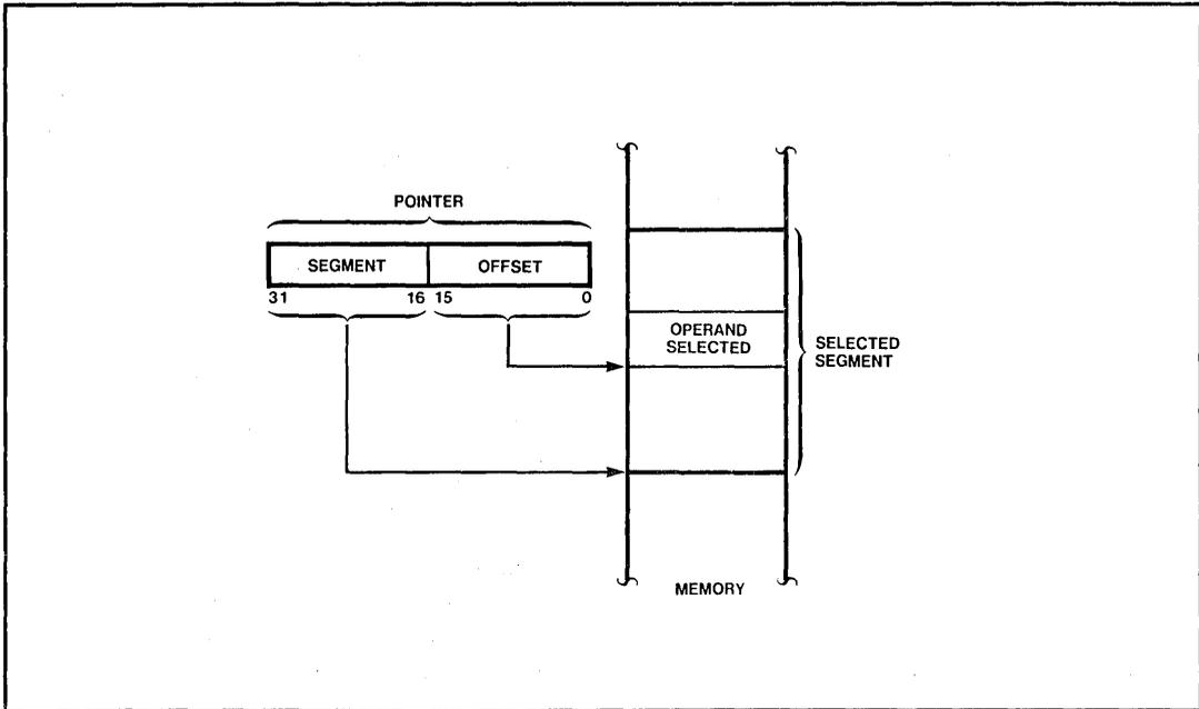
Figure 2-11. Two-Component Address
