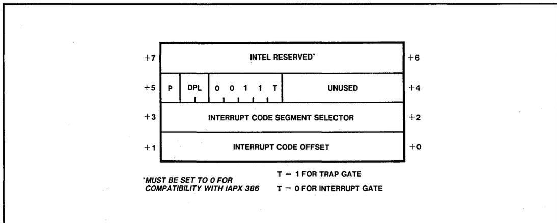
**Figure 9-3. Trap/Interrupt Gate Descriptors**
