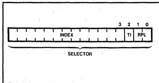
Figure 6-2. Format of the Segment Selector Component
