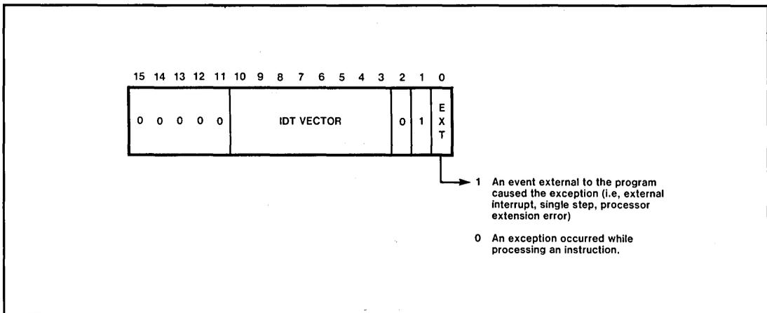
Figure 9-2. IDT Selector Error Code
