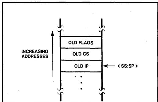
Figure 5-4. Stack Structure After Interrupt (Real Address Mode)
