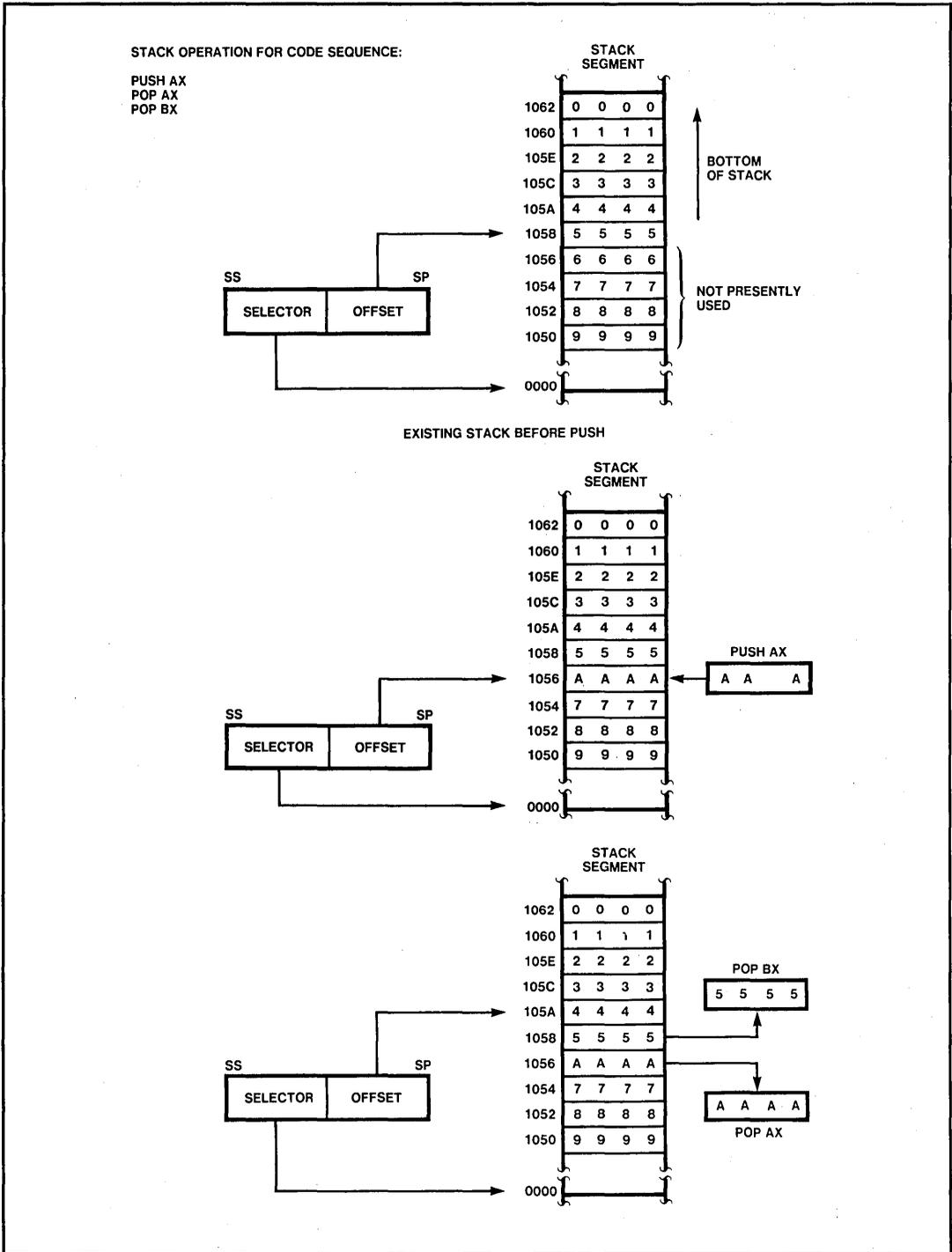
Figure 2-8. Stack Operation
