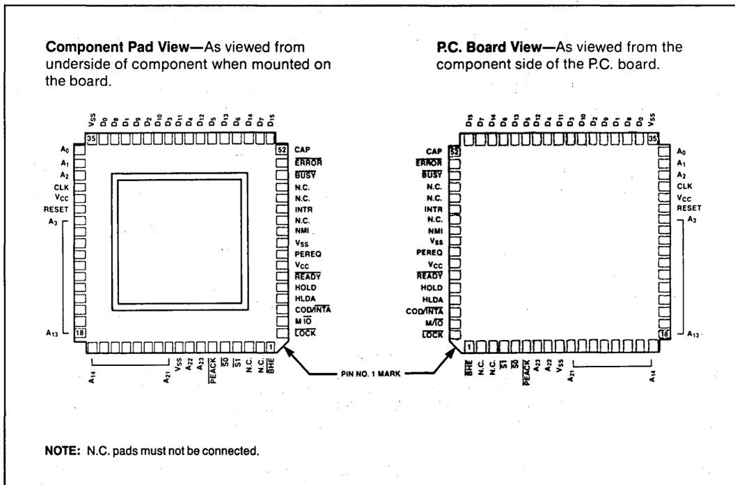
Figure 2. 80286 Pin Configuration
