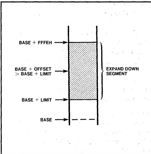
Figure 11-1. Expand Down Segment
