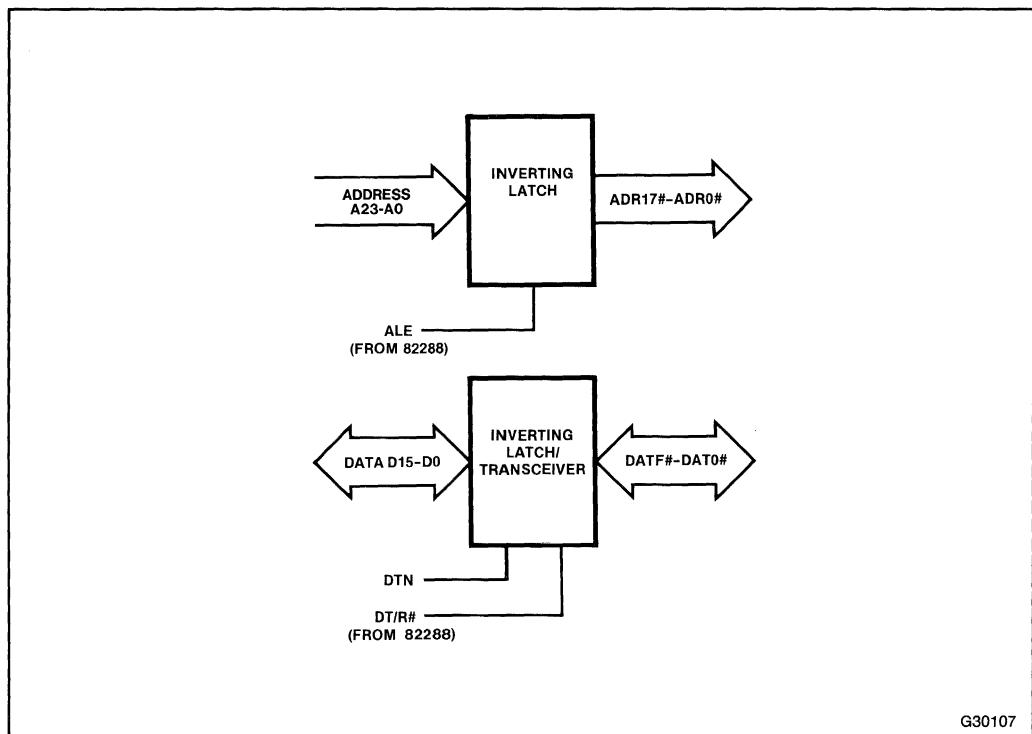
Figure 9-2. MULTIBUS® I Address Latches and Data Transceivers
