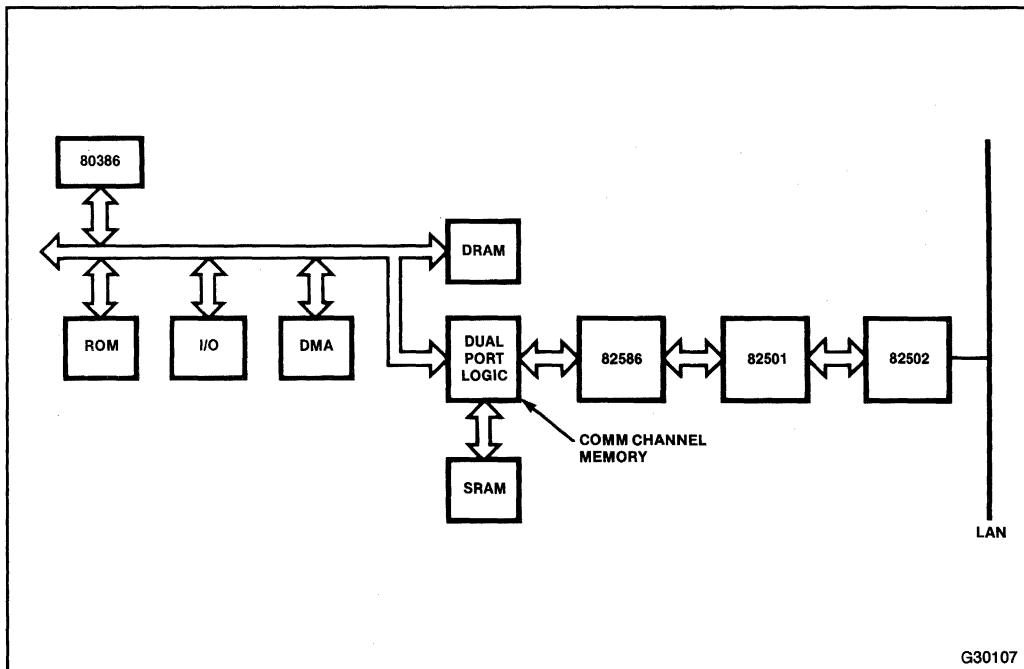
**Figure 8-16. Decoupled Dual-Port Memory Interface**
