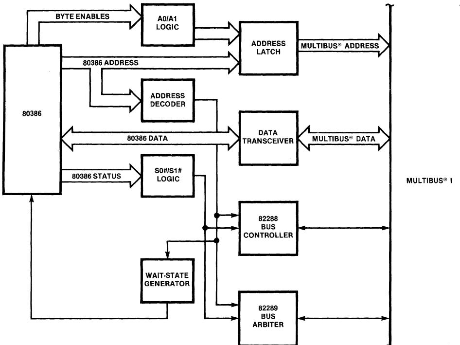
Figure 9-1. 80386-MULTIBUS® I Interface
