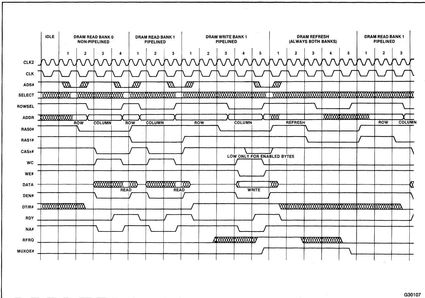
Figure 6-9. 3-CLK DRAM Controller Cycles
