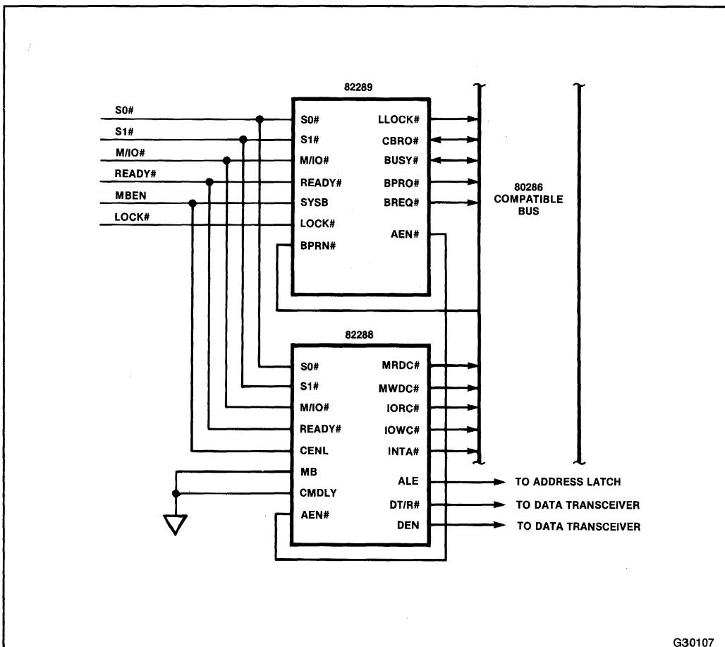
Figure 8-12. 82288 and 82289 Connections
