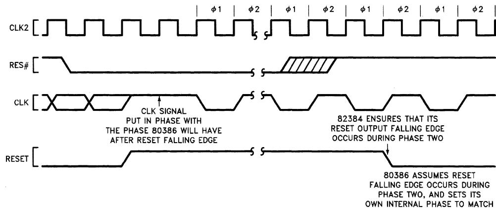
Figure 3-21. RESET, CLK, and CLK2 Timing
