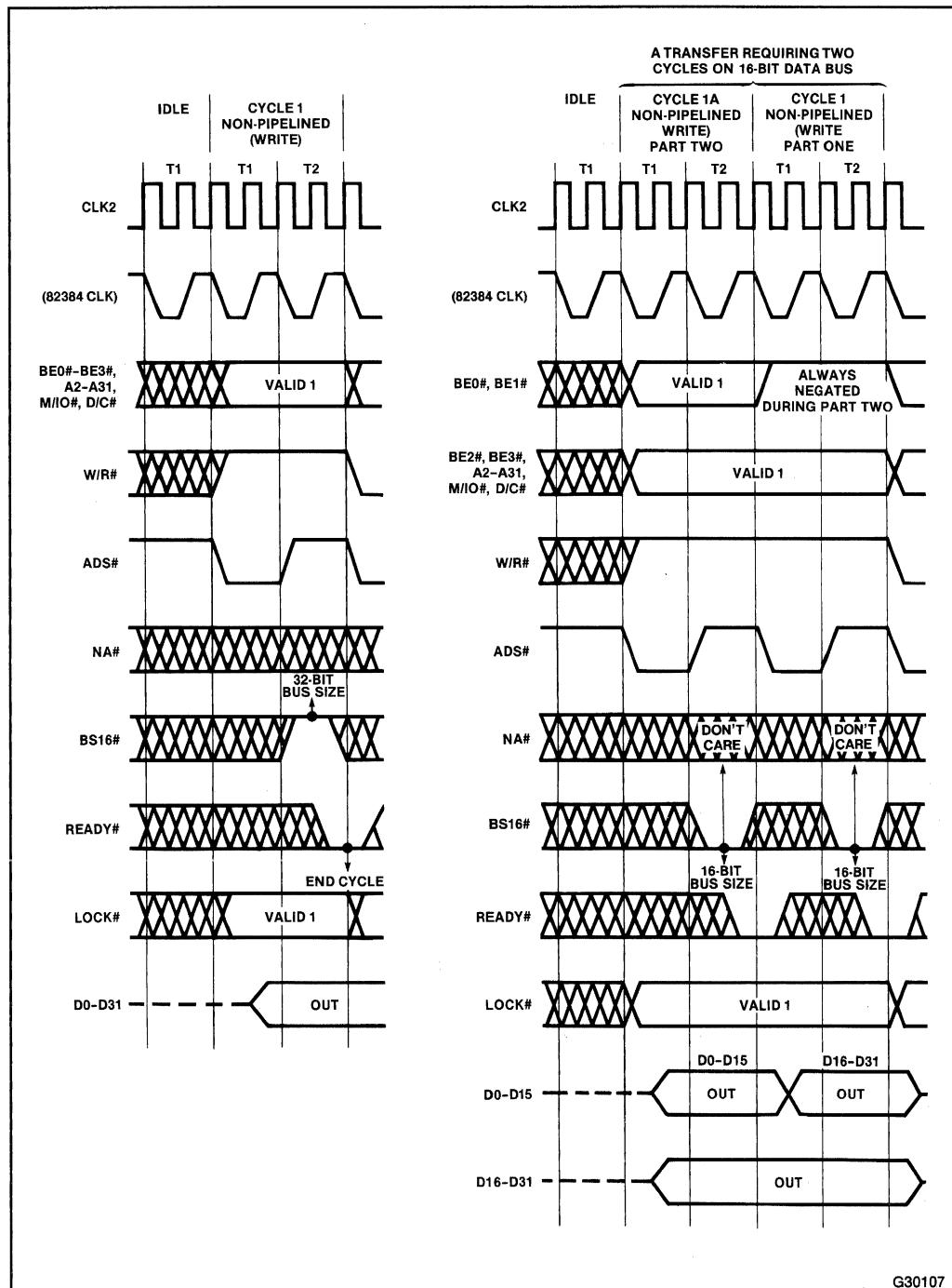
Figure 3-13. 32-Bit and 16-Bit Bus Cycle Timing
