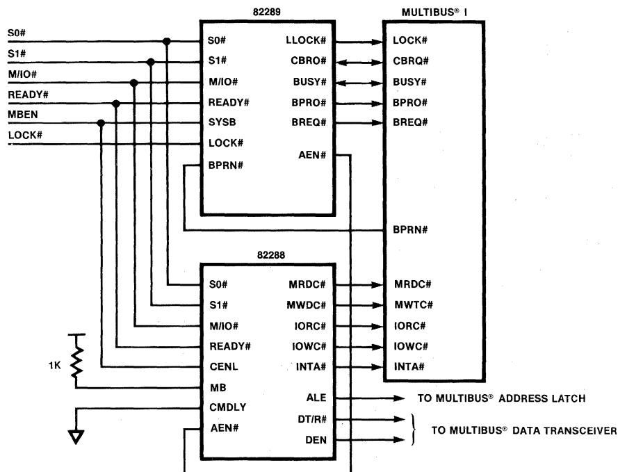
Figure 9-4. MULTIBUS® Arbiter and Bus Controller
