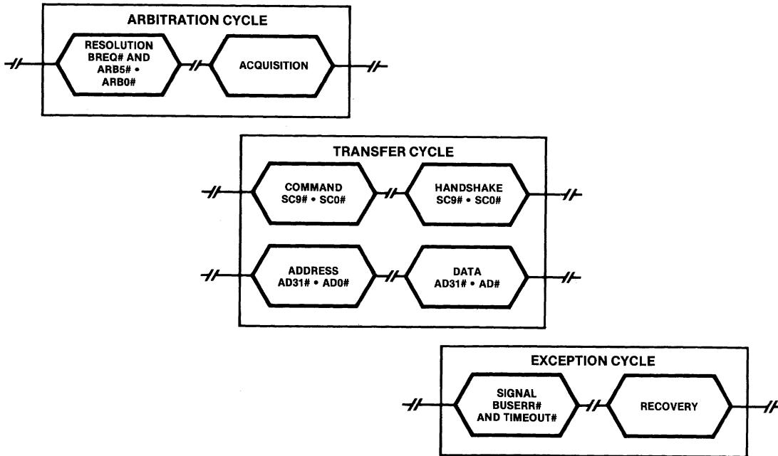
Figure 10-1. iPSB Bus Cycle Timing
