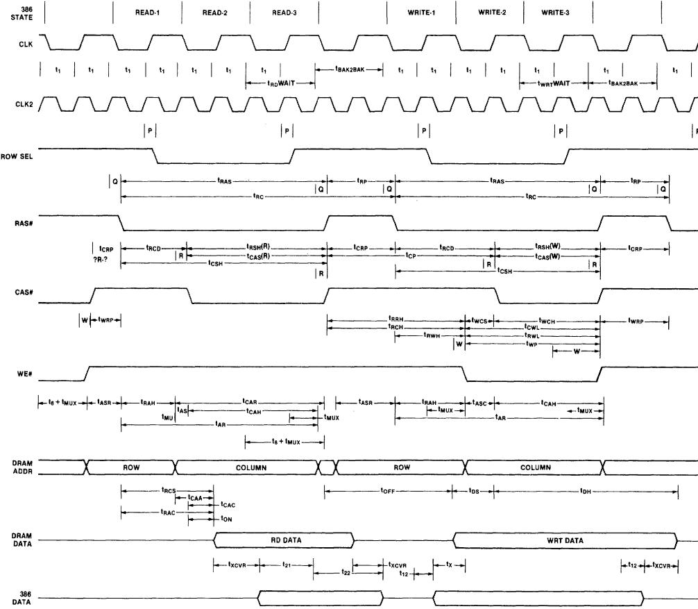
Figure C-8. DRAM Circuit Timing Diagram
