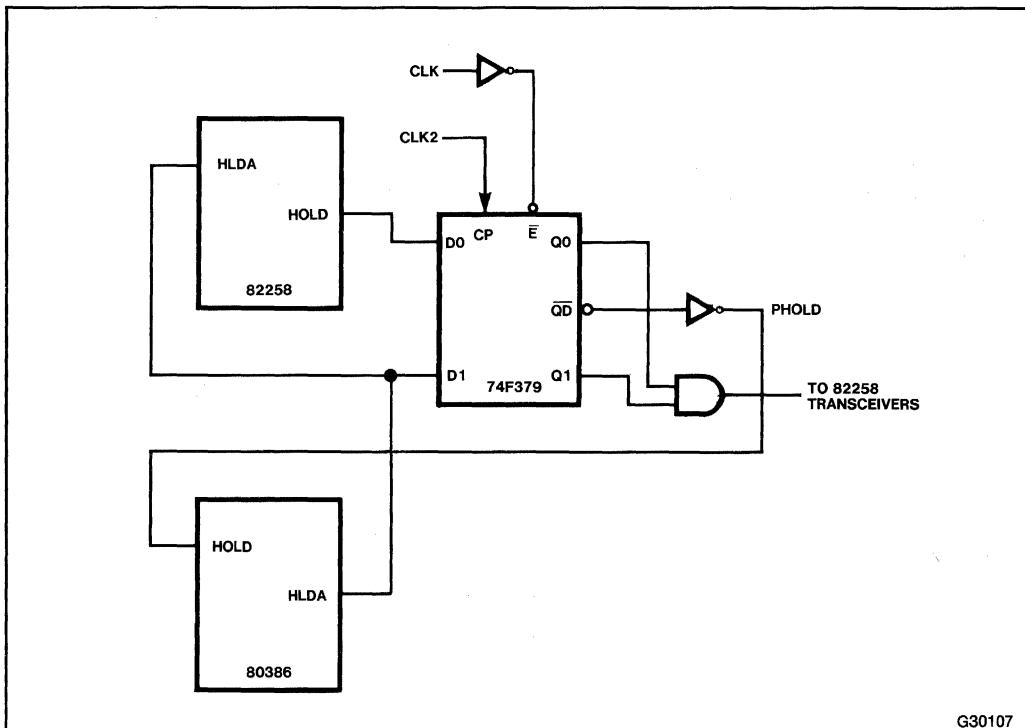
Figure 8-13. HOLD and HLDA Logic for 80386-82258 Interface
