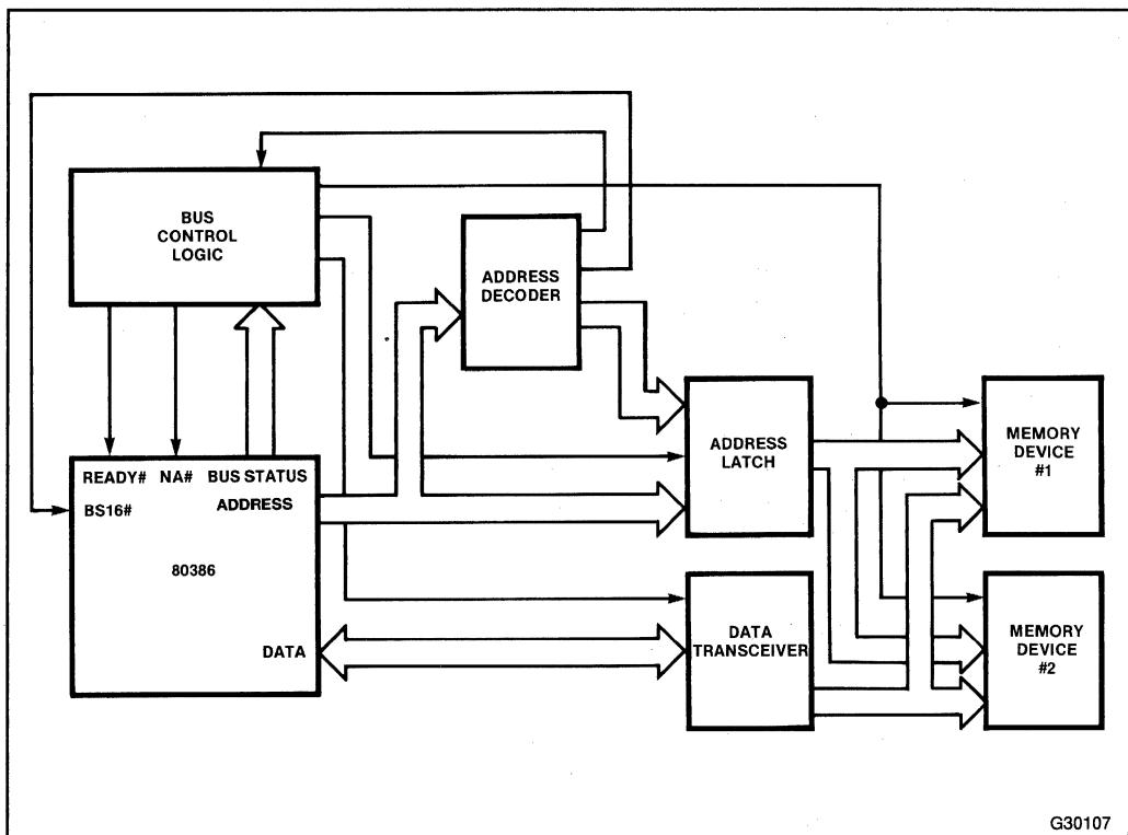
Figure 6-1. Basic Memory Interface Block Diagram
