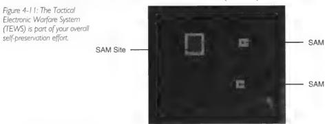
The Tactical Electronic Warfare System (pronounced "Tooz") is an integral part of your aircraft's self-defense capability. It consists of an array of sophisticated sensors and receivers located throughout the aircraft. The TEWS gives you the ability to locate enemy aircraft by the energy their radars emit. It also allows you to pinpoint the location of ground based tracking radars. In fact, any radar that is emitting energy, whether it be friend or foe, is detectable.
