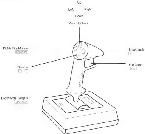
FLIGHTSTICK PRO™ consists of four main components; a standard pistol grip joystick, a four-position hat controller, a wheel type throttle control and four control buttons/switches.
