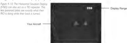
By pressing the HSD/TID Toggle Snift R the HSD monitor is turned into a TID repeater. This way, you can see all the information currently showing up on the RIO's TID. The range (in nm) of the display is shown in the upper right hand corner of the monitor.
