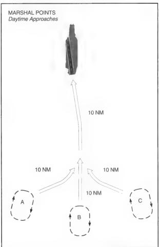
Figure 3-10: When your landing is delayed the ATC will send you to a holding area known as a Marshal Point.
