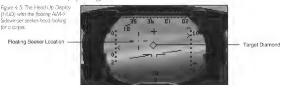
By pressing the Sidewinder 2, the HUD symbology is changed to reflect that your AIM-9 heat-seeking Sidewinder missiles have been placed in priority.
