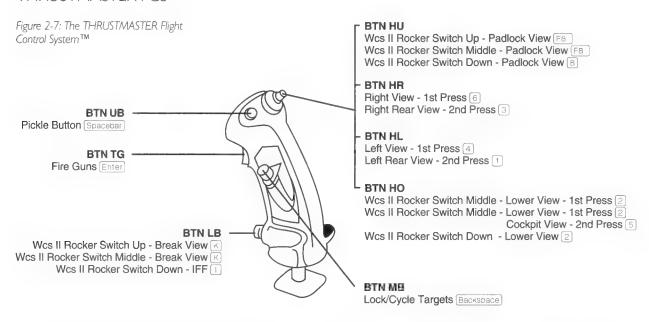
The THRUSTMASTER Flight Control System<sup>™</sup> is compatible with *FLEET DEFENDER*. It consists of three main components, a pistol-grip flight stick, a four-position *hat* controller, and four control buttons. These controls (or combination of control buttons) emulate keyboard functions as shown in the diagram.
