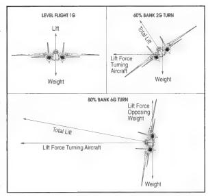
Figure 3-3: G-Forces when banking. As you can see the flight attitude (bank angle) that an aircraft assumes while turning has a direct relationship to the number of "G's" inflicted on the aircraft and pilot.
