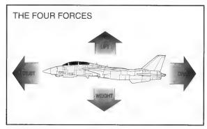
Figure 3-1: As you can see by the above diagram the laws of physics act and counter-act upon an aircraft. Controlled flight is merely the art of juggling these four forces.
