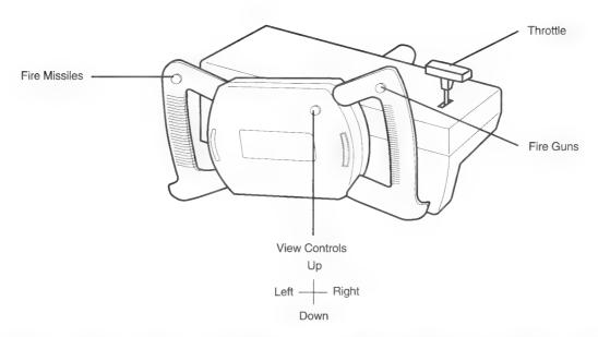
VIRTUAL PILOT™ consists of four main components; a steering wheel device, a four-position hat controller, a bar throttle control and four control buttons/switches.
