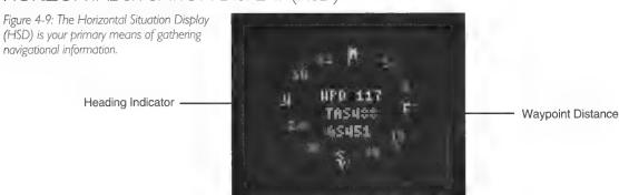
The Horizontal Situation Display (HSD) consists of a rotating compass dial with three lines of navigational text information inserted in the center. Like the VDI, it is multi-functional. This monitor can alternate between showing standard HSD navigational information and being a Target Information Display (TID) repeater.
