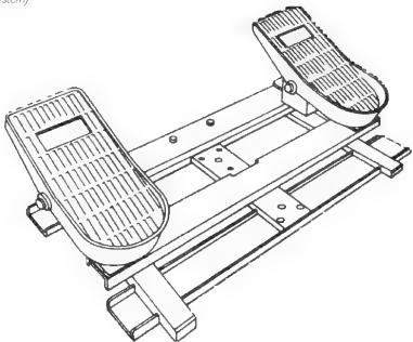
The THRUSTMASTER RCS™ (Rudder Control System) consists of two linked foot pedals which operate the aircraft's rudders. Moving the foot pedals, forward and back, emulates the Rudder Left , and Rudder Right .
