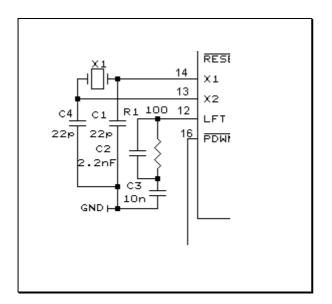
Note : the X2 output cannot be used to drive another circuit.
