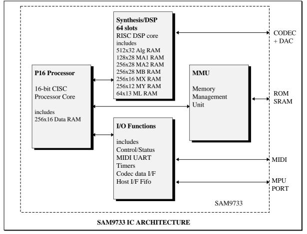
The SAM9733 is a low cost derivative of the SAM9407 and SAM9503. It retains the same high quality synthesis with up to 64 voices polyphony. The SAM9733 maximum wavetable memory is 4 megabytes and the ISA bus communication is through a standard MPU-401. The SAM9733 is packaged into an industry standard 100 pins plastic quad flat pack (PQFP100)
