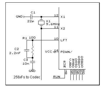
Note : If the X2 output is not used as a Codec clock, then an additional 22pF capacitor from X2 to GND should be implemented.
