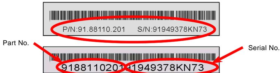
**P/N: 91.88110.201** is part number, **S/N: 91949378KN73** is serial number.
